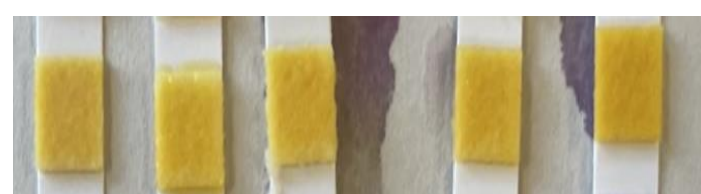
Figure 4. Lead test strips Pb concentration: (left to right): 0, 500 0.5, 1.5, 3.0, 4.5 ppb
