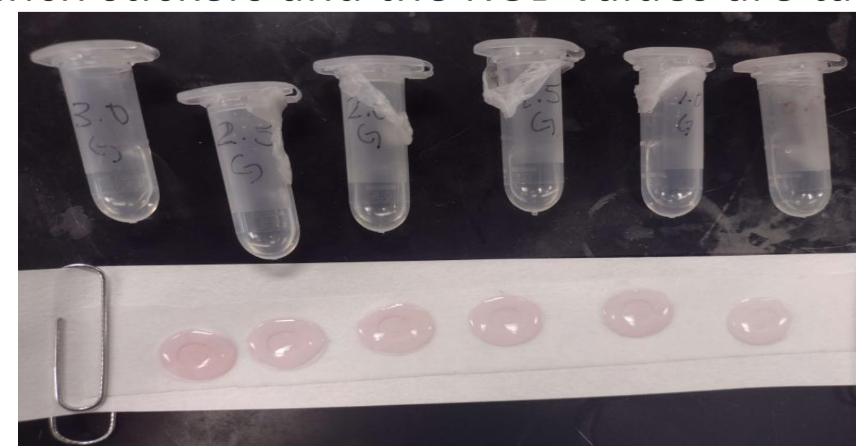
Figure 1. 0.5mg/ml to 3.0mg/ml concentrations with color reagent on wax paper on top of chromatography paper.
